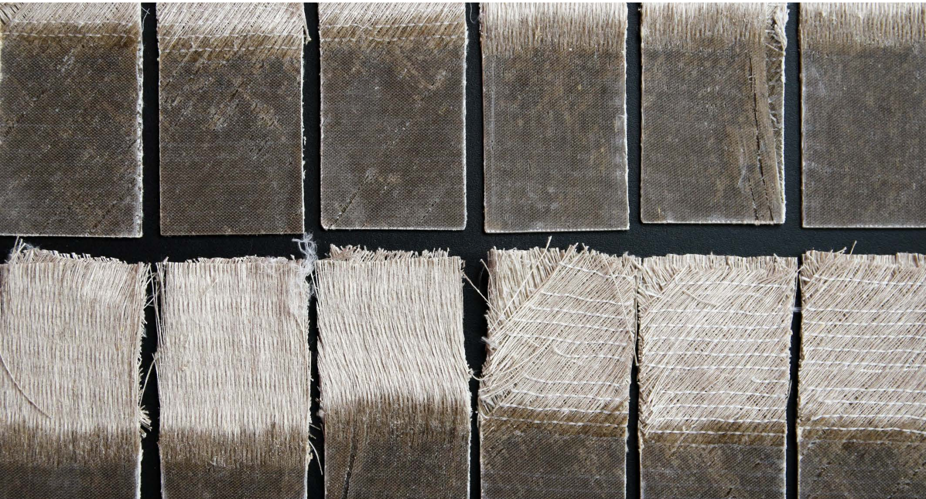
Different types of non-crimp flax fabrics
